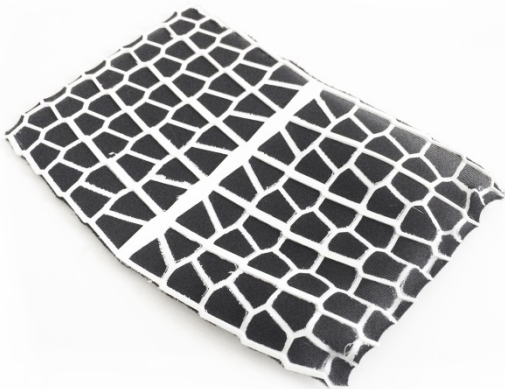
Fig.09. 3D printed pattern with three different edge dimensions
