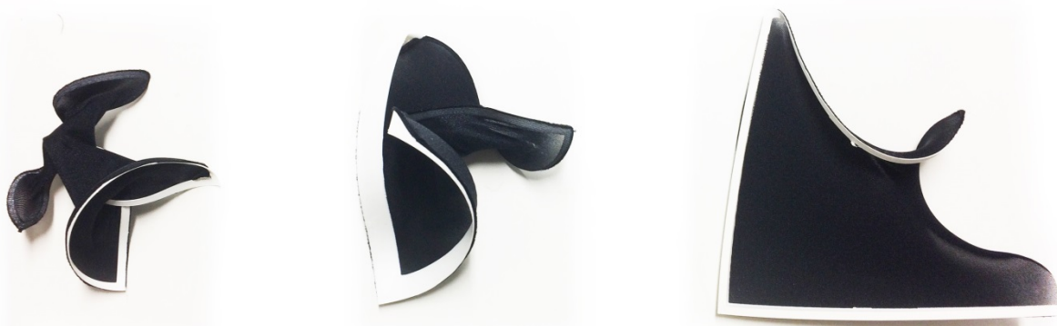
Fig.06. Three modules of 18,5 x 18,5 cm each with various 3D printed edge thickness (left: the same thickness of all the four edges: W: 5mm, H:0,6mm , middle: two edges W: 5mm, H:0,6mm and two wider ones: W: 15mm, H:0,6mm, right: 2 edges W: 5mm, H:0,6mm and two higher ones: W: 5mm, H:8 mm)
