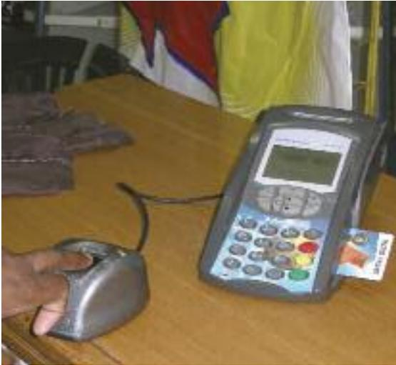
**A Point of Sale device with an electronic finger print reader being used by a shop keeper to authenticate the identity of a recipient of child benefit in South Africa.**
