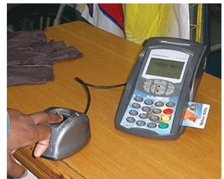
A POS device with an electronic finger print reader being used by a shop keeper to authenticate the identity of a recipient of child benefit identity in South Africa.
