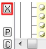
This "X"-button can be enabled in the CCU Supervisor Module under the menu-option "Internal Tables", "Users". Over here, you open the user which needs this button and click the sheet "Autorization". The authorization that needs to be enabled (checked) is "Copy/Cut all linked articles". After this is done, the user should restart CCU to actually see this.
