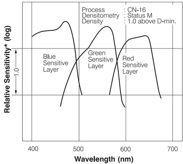
\* Sensitivity equals the reciprocal of the exposure (J/cm<sup>2</sup>) required to produce a specified density.
